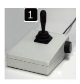
Tilt the lever of the joystick to move the stage toward you.
