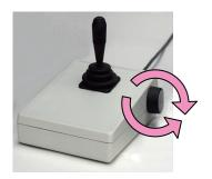
1 Set the focus using the joystick focus dial.
